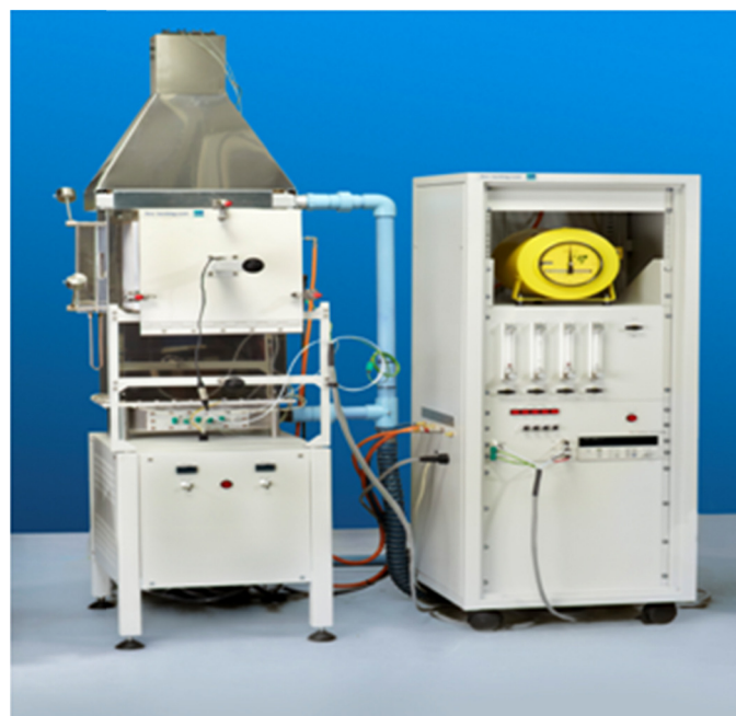
Fig. 8. Ohio State University heat release (OSU) apparatus.
