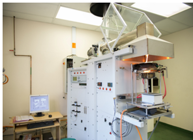
Fig. 3. Cone calorimeter apparatus (from the Council for Scientific and Industrial Research (CSIR) fire testing laboratory).
